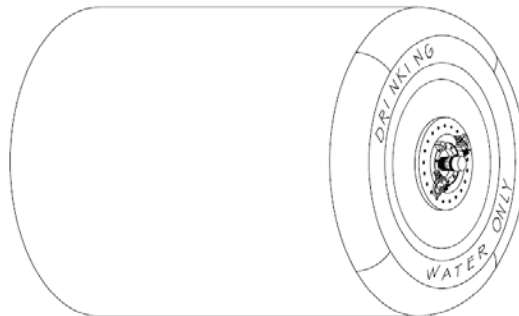
Figure 1. The 500 Gallon Water Drum.
